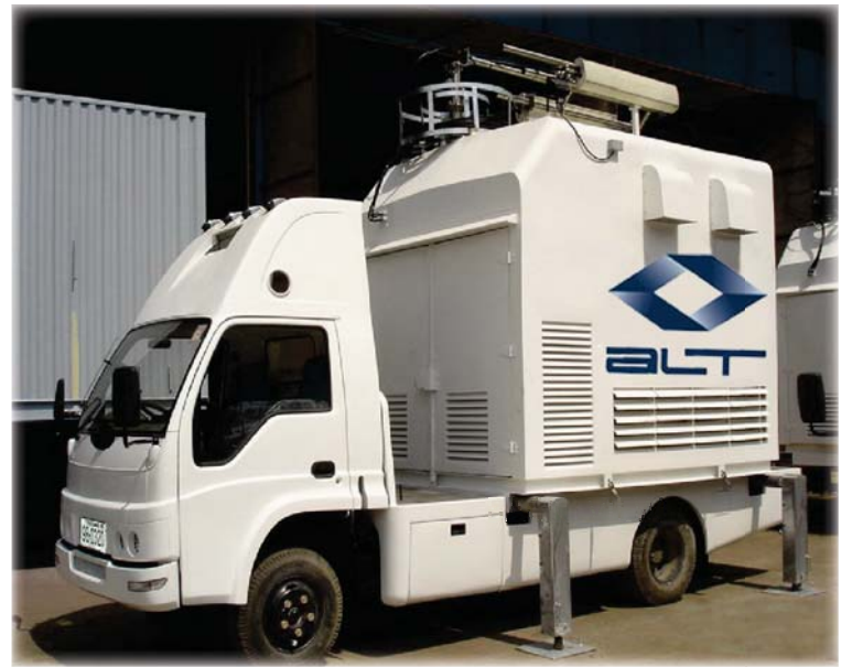
Outdoor Enclosure installed on platform (4 legs)
